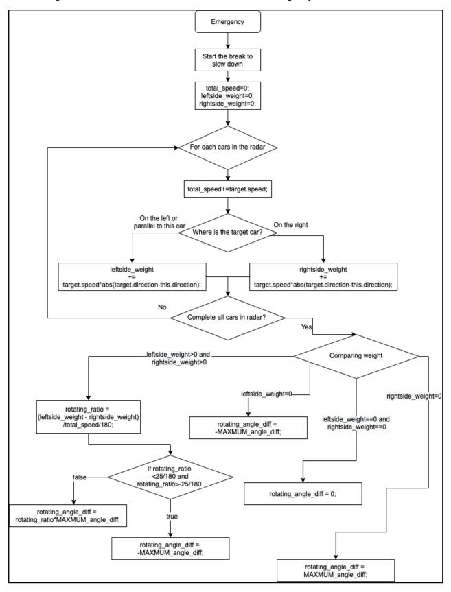
5.2 Algorithm Flow Chart of Cars in simulator under Emergency status
